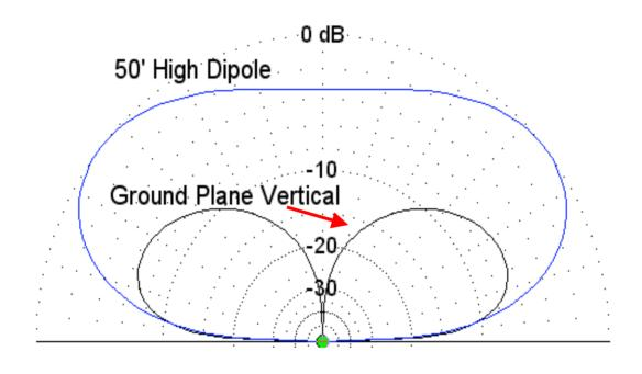
Over "typical" soil, a vertical will lose out to a 50-foot high horizontal dipole.
