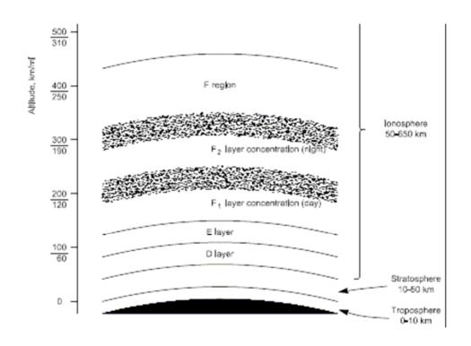
Solar excitation of trace elements creates ionized regions: D, E,  $F_1$  and  $F_2$ . The  $F_2$  region is the most important for long-distance HF communications.
